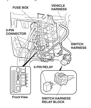
39. Plug the switch harness 5-pin connector into the 5-pin slot of the fuse box.
