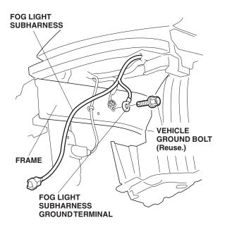
19. Secure the fog light subharness to the vehicle frame and panel hole using the two wire ties with clips at the green-taped locations.
