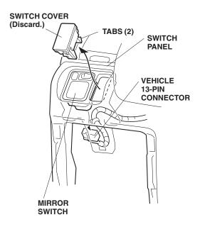
43. Plug the switch harness 13-pin connector into the mirror switch. Plug the vehicle mirror switch 13-pin connector into the switch harness 13-pin connector.
