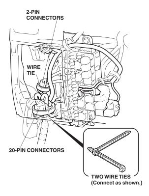
50. Secure the 2-pin connector to the vehicle harness with one wire tie.
