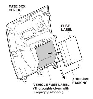
37. Remove the adhesive backing from the fuse label, and then attach the fuse label over the existing vehicle fuse label as shown.
