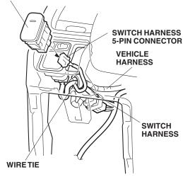
45. Secure the switch harness to the vehicle harness with one wire tie.
