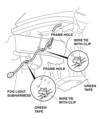
20. Secure the fog light subharness to the vehicle harness with three wire ties.
