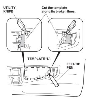
9. Using a felt-tip pen, mark the front bumper along the outer edge of the template. Remove the template.
