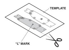
6. On the outside of the front bumper, place the left template along the front bumper and tape it in place.
