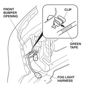
24. Route the fog light harness along the front bumper to the right side of the vehicle and attach the five fog light harness clips to the five ribs inside the front bumper.
