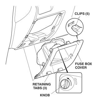
36. Using isopropyl alcohol on a shop towel, thoroughly clean the vehicle fuse label on the back of the fuse box cover.
